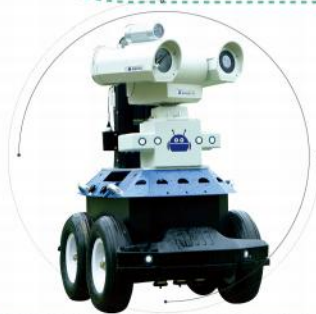
Substation inspection equipment
