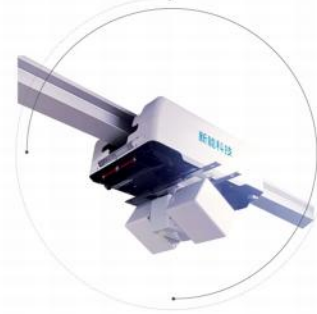
Cable tunnel inspection robot
